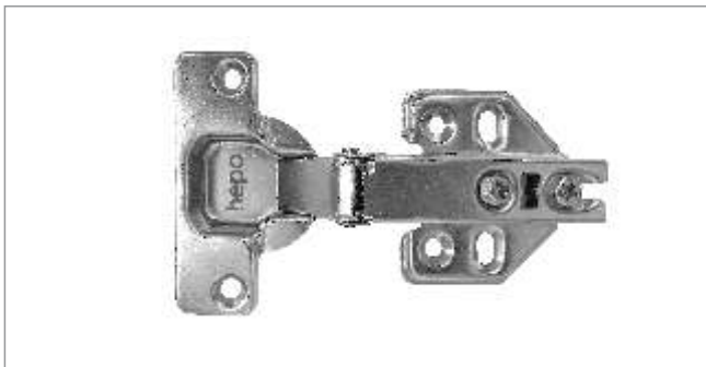
Reliable Concealed hinge: Auto Close & Integrated Soft Close With Auto close as well as with Integrated Soft close feature Tested & Certified for 20,000 Cycles & 24 hrs Salt Spray
